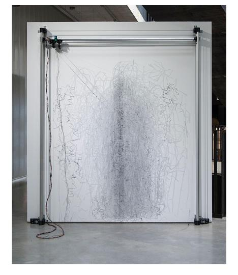
Unerasable traces of you, 2023 250 x 200 cm Handbuilt pen plotter: Aluminium rods, 3D printed parts, Wires, Arduino, Cnc v3 shield, computer, motors, GT2 belts, screws
